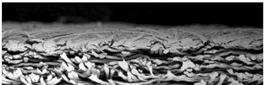
*Three dimensional medias (above) have depth loading properties while two dimensional medias (below) are typically surface loading.*
