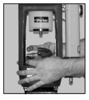
3. Using a molybdenum disulfide type grease, apply a thin layer of grease to the die bowl.
